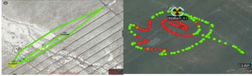
Figure 1-1: Aerial UAV Radiation Mapping. Including a mapping mission with 2 UAVs searchign an area over 1 km away (left). The other is a smaller scale mapping test at Briggs Field at MIT in which the contour pattern is more easily visible (right). Both using real radiation sources of 7.8 mCi ^{137}\text{Cs} (right) and a mixed source totalling approximately 98 mCi of mostly ^{60}\text{Co} (left).
