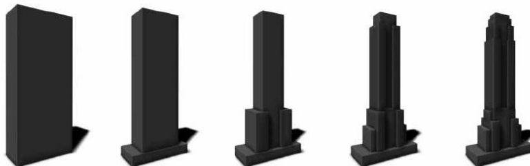
Figure 2.1.2. Generation of a building using an extended L-system, as presented in (Parish & Muller, 2001).
