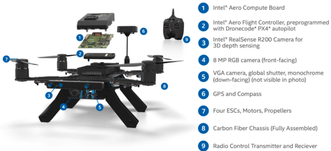
Figure 2-1: The Intel Aero Ready to Fly drone components (figure in courtesy of [19]).
