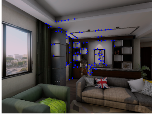
Figure 4-5: Features chosen by the K-Fastest method
