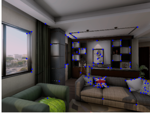
Figure 4-4: Features chosen using the quality metric of GoodFeaturesToTrack
