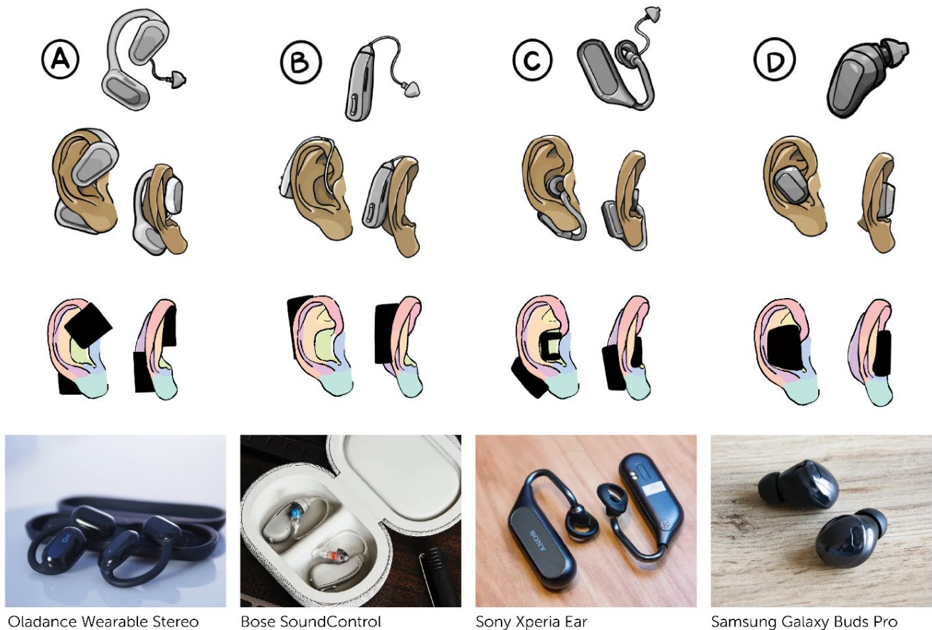
Figure 3: Four devices were presented to survey takers to discuss. (Row 1) Perspective drawing of the device with their respective letter label (Row 2) The devices from different angles on the ear (Row 3) A visual mapping of where the device interfaces with the ear surface (Row 4) The respective reference product that the device was based on.
