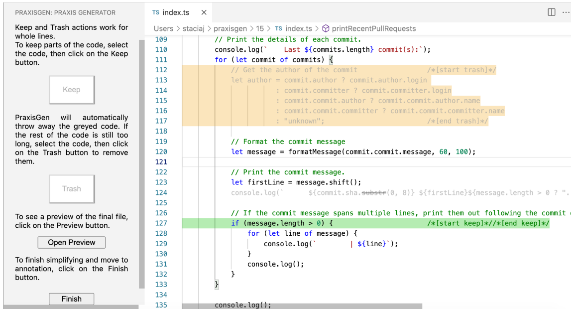
Figure 3-8: A view of PraxisGen Simplify. Code that is highlighted green indicates that the code is Kept, and code that is highlighted orange indicates that it is Trashed.
