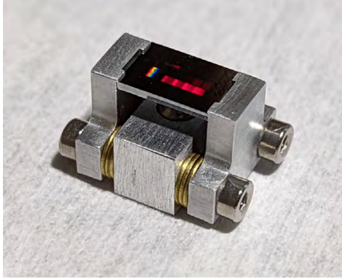
Figure 3-10: Sample mount with set pin to flatten stress-buckled suspended membranes.
