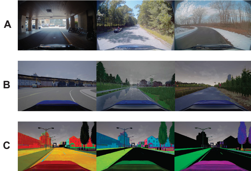
Figure 3-7: Training images from various comparison methods. Samples drawn from the real-world ( IMIT-AUG ; A) and the model-based simulator CARLA (B-C). Domain randomization ( DR-AUG ; C) illustrates transformations of a single location for comparison.
