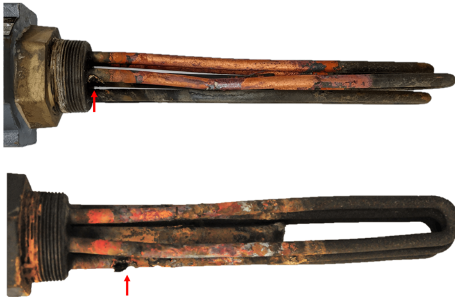
(b) Holes observed at approximately 1 cm and 5 cm from the heater's base.
