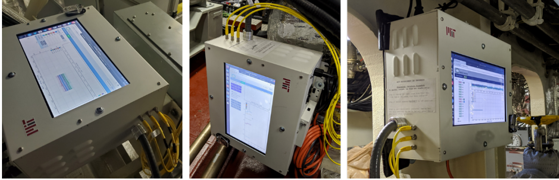
Figure A-5: NILM installs on USS Indianapolis (LCS 17).
