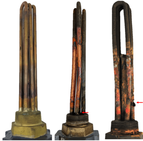
(b) New heater and degraded heaters with holes 1 cm and 5 cm from base, respectively.
