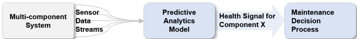
Figure 2-1: Some systems have many sensors that provide data while the system operates. This data can be used in predictive analytics tools and models to predict the health of different components on the system. The output of a predictive analytics model is a health signal, which is an input to the maintenance process.
