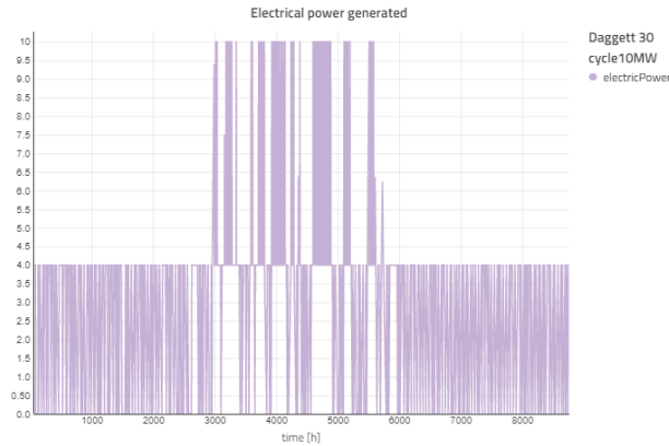
Figure 4-2: Profile of electrical power generated by a 10 MW e plant in Daggett, CA so the heliostat area required for this location’s 10 MW e plant to achieve a 30% CF is low. With a low heliostat area, the plant actually operates at nominal power output (10 MW e ) for only a small fraction of the year, mainly in the summer. The rest of
