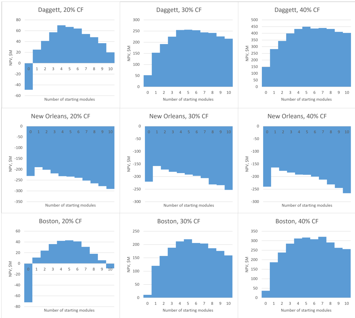
Figure 4-13: Bar graphs for each of the 9 cases showing how the number of starting modules affects the stochastic ENPV of the modular approach.
