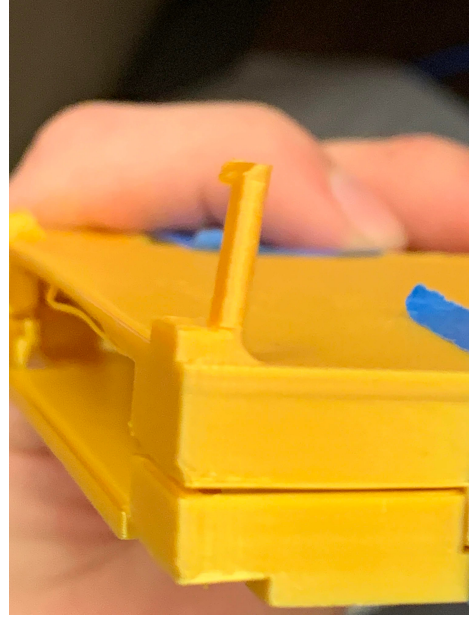
(b) A fracture on the base of a cantilever, as shown from the back.
