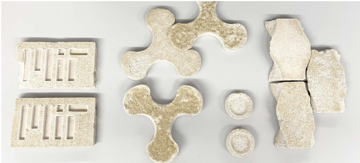
Figure 26 Biocementation Results: Biocemented modules and objects using PLA molds.
