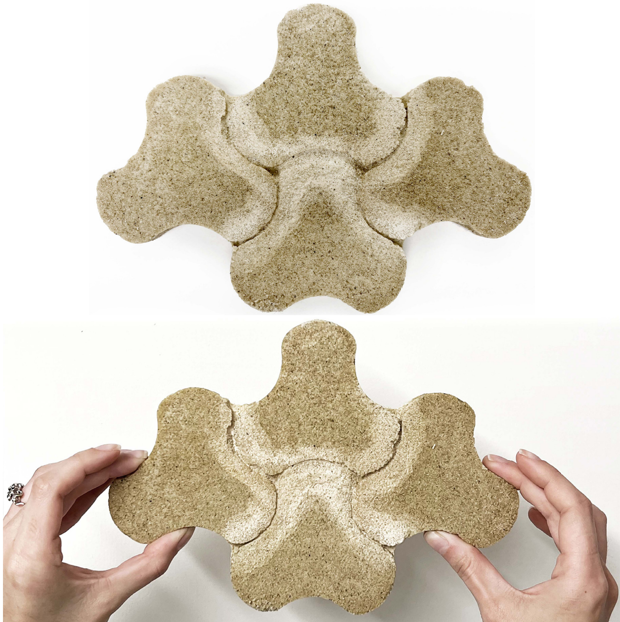
Figure 34 Biocemented Assemblies: Four units joined together with biocement. The areas that received extra rounds of biocement have begun to turn white.
