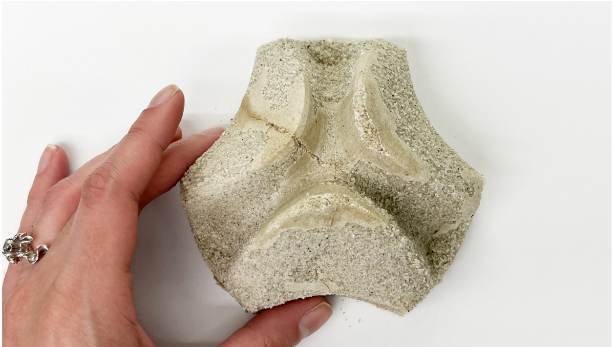
Figure 29 Casted Module: Biocemented three-dimensional module.
