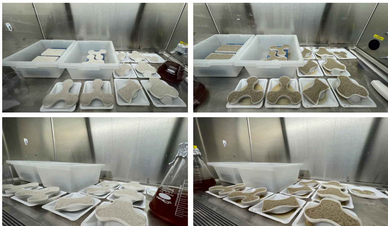
Figure 25 Biocementation: Biocementation process occurring in the biosafety cabinet. PLA molds filled with coarse sand (Left) and inoculated with bacteria and biocement solution (Right).
