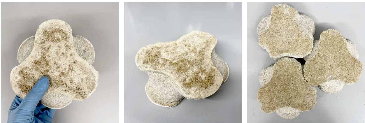
Figure 27 Interlocking: Biocemented interlocking modules.
