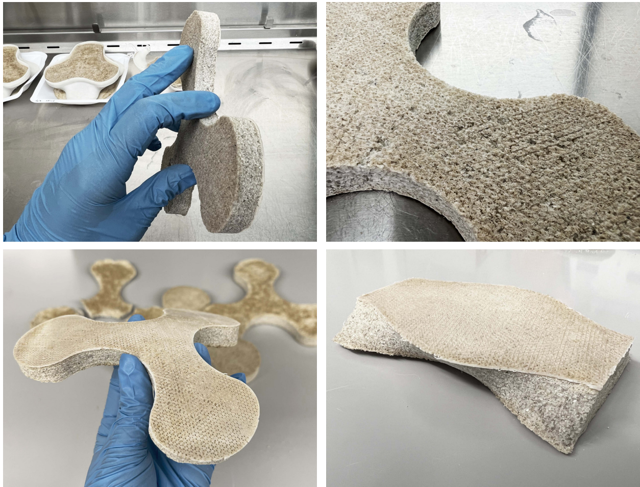
Figure 28 Resolution and Bonding: Biocementation results including crisp edges (Top Left), high resolution (Top Right), curvature from bowing formwork (Bottom Left), and bonding to the PLA (Bottom Right).
