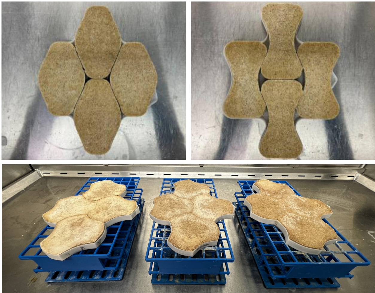
Figure 33 Biocementation: Tiles placed within 3D printed PLA molds to prevent movement while joining (Top) Biocemented tiles in molds (Bottom).
