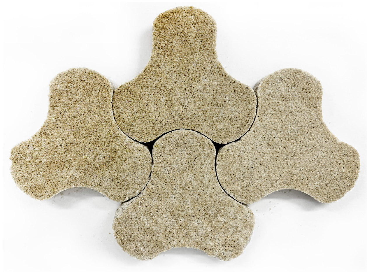
Figure 31 Tiles to be Assembled: A group of modules ready to be biocemented together.
