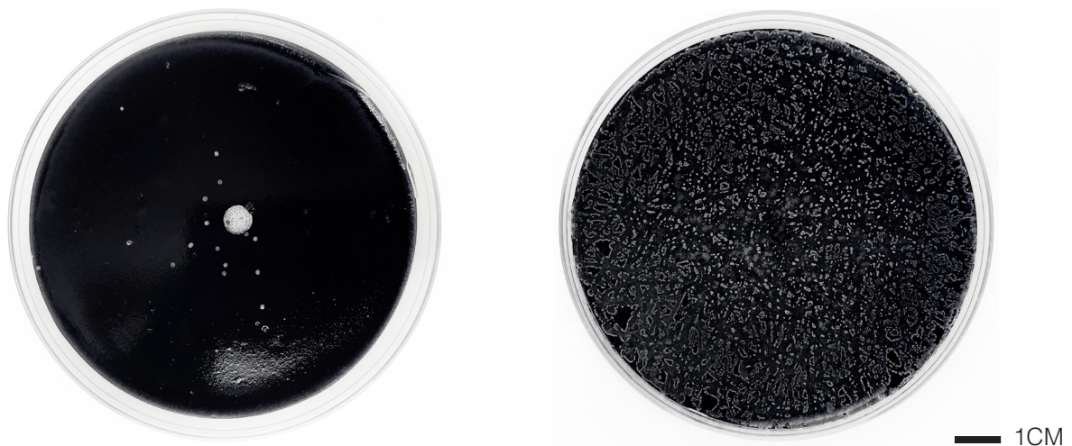
Figure 12 Localized Calcification: Petri dishes with S.pasteurii demonstrating local calcification effects. Microbes centrally deposited (Left) Microbes distributed evenly across surface (Right)
