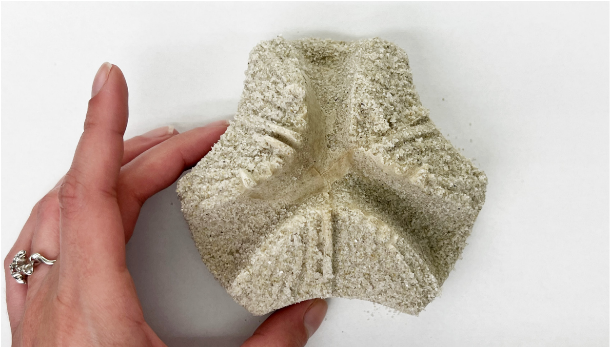
Figure 30 Casted Module with Grooves: Biocemented three-dimensional module with grooves.
