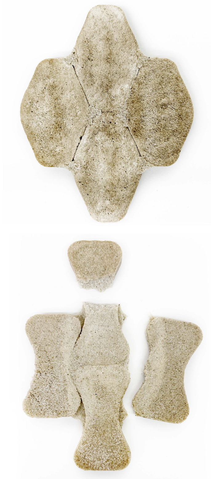
Figure 35 Biocementation of Various Assembly Geometries: Different biocemented geometries including a convex hexagon (Top) and a concave hexagon (Bottom) were tested.
