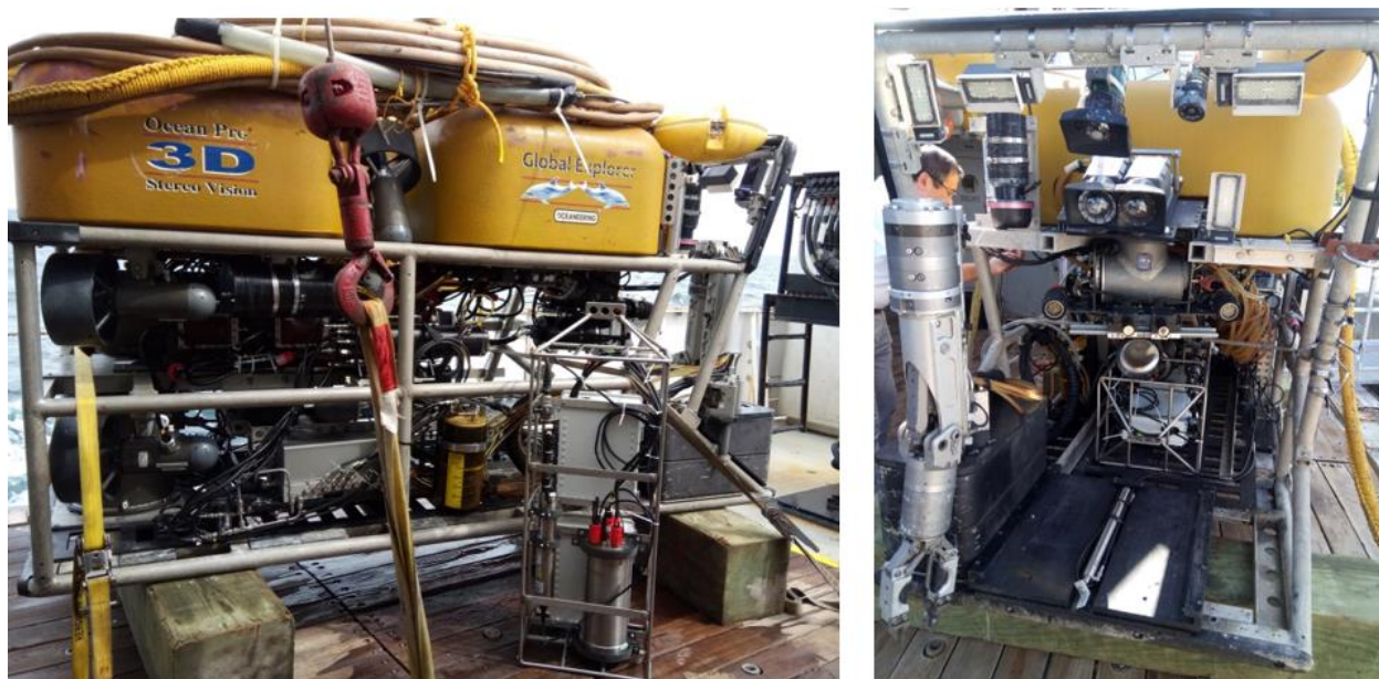
Figure 3.2: CHANOS II on ROV Global Explorer . The sensor is mounted in the belly of the ROV to allow the inlet to be as close to the seafloor and coral mounds as possible.
