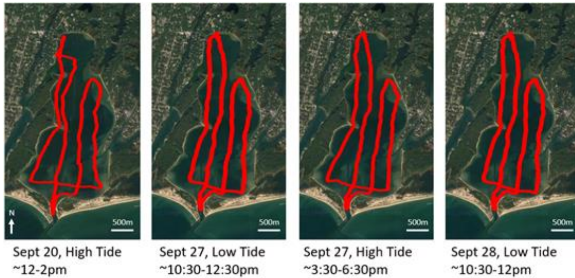
Figure 2.17. Underway towing transects at Waquoit Bay as recorded by GPS trackers carried on the Trifly . Individual transects vary slightly due to sandbars and local boat traffic.
