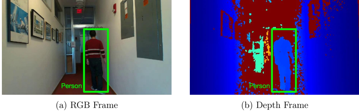
Figure 6-3: Target localization with the ground-truth LiDAR camera. To extract the ground truth, we apply a computer vision person detector to the RGB frames and use the depth of the pixel in the detected region (the green rectangle) to compute the ground-truth location of the target.
