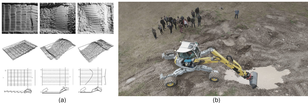
Figure 12: (a) “Feedback driven design explorations by students Ladina Ramming and Thorben Westerhuys” (b) HEAP autonomous walking excavator (Hurkxkens et al. 2020)
