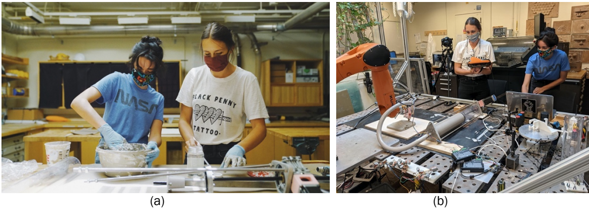
Figure 29: (a) Mixing clay to load extruder, and (b) experimental set-up
