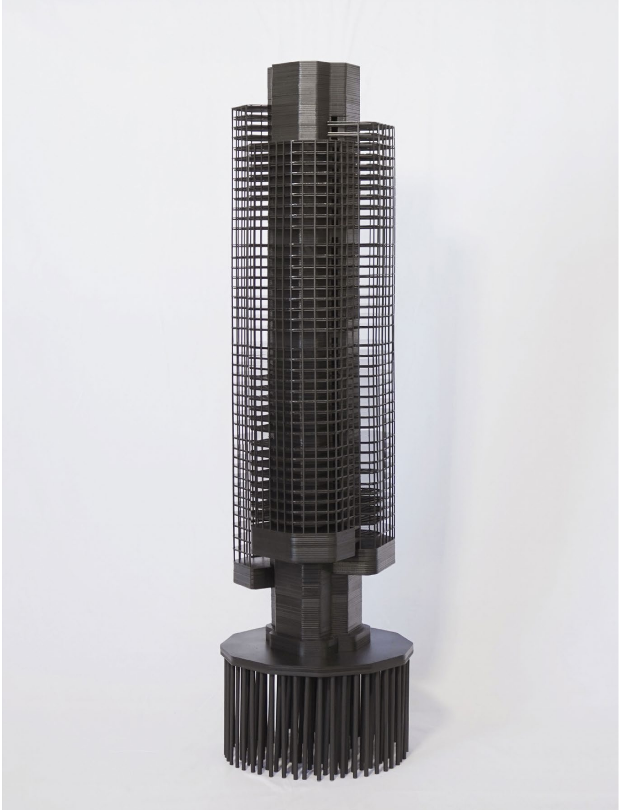
Fig 03: Tower 42 - Structural Model (1:200)
