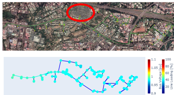
Figure 4-1: GIS and low flow result of distribution network serving the Wuse Market (highlighted in red).
