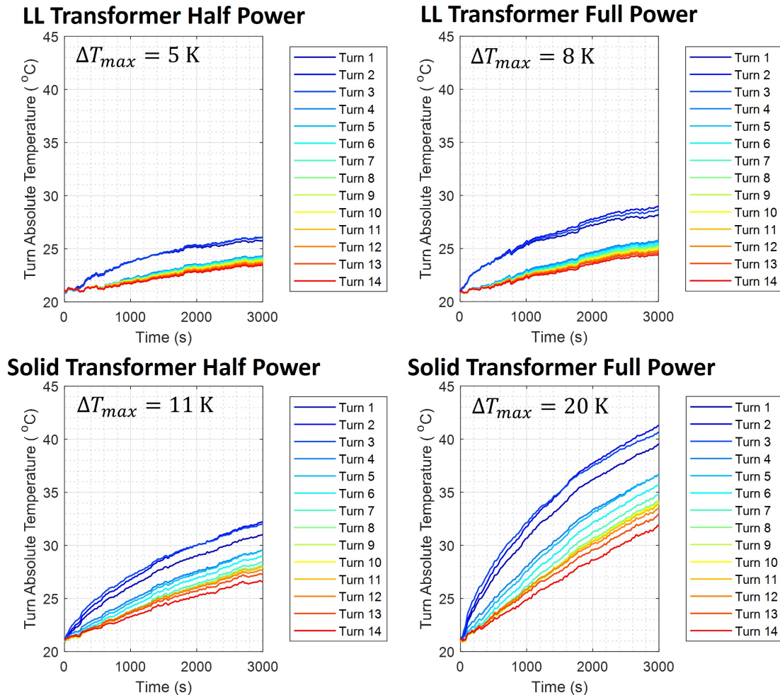
Figure 4-14: Temperature vs. time profile for the two transformers (Low Loss = LL) operated at full (1.5 kW) and half (750 W) power for 50 minutes. The maximum temperature rise, amongst all observable turns, from the start to end of the 50 minute window is shown.
