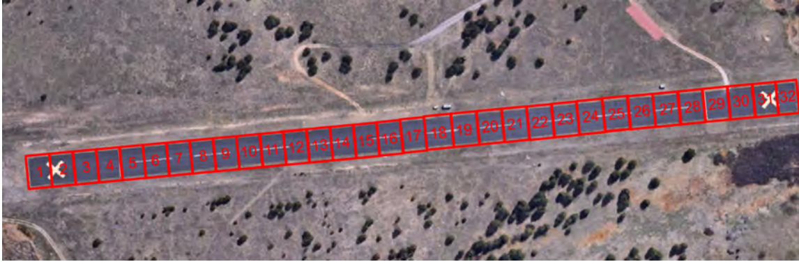
Figure 4-5: The Aardvark runway is divided into 32 sample units for the purpose of PCI inspection.
