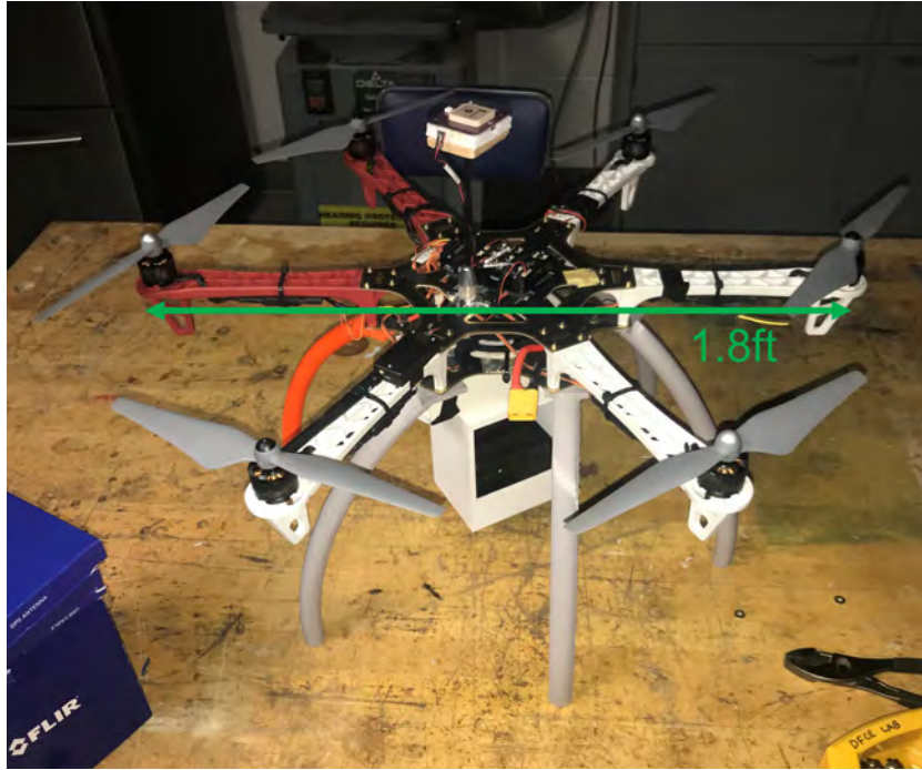
Figure 4-3: The drone used to image the airfield in this study is shown above, having a propeller-to-propeller length (also called "wheelbase") of 1.8ft.
