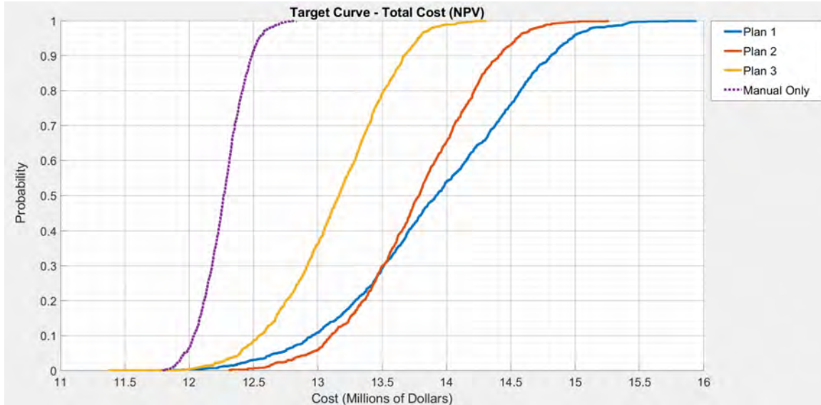
Figure 5-3: These cumulative distribution functions correspond to the distributions of total costs produced by a thousand interactions of Monte Carlo simulation. Each of the curves correspond to a different implementation strategy. Because cost in term of NPV is represented on the horizontal axis, lower values and distributions shifted left are desirable.
