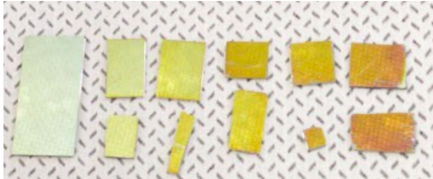
Figure 18: Photograph of the ITO on silicon samples used in ellipsometry measurements. From left to right, we see a non-reduced sample, then samples reduced for 60, 90, 120, 150 and 180 s. Though the samples have already been subdivided for other experiments by this photo, the upper and lower samples represent the “a” and “b” reductions, and they were all originally the same size and shape.
