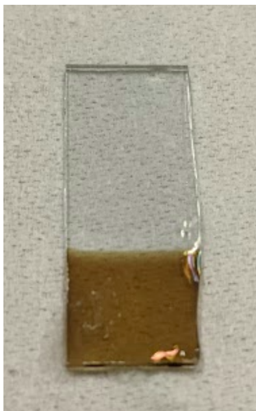
Figure 7: A photograph of ITO on glass, the lower half of which was exposed to about 75 \text{ mC/cm}^2 reduction charge density.
