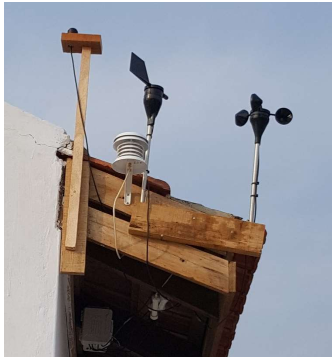
Figure 20: Bhuj, India weather station. From left to right: Solar radiation sensor, Temperature/RH sensor in solar shield, wind direction sensor, and wind speed sensor.
