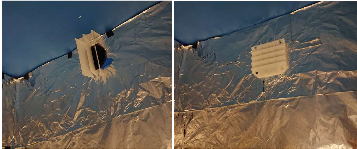
Figure 44: Inlet Louvers. 1" Offset (Left) and 4.2" Offset (Right)
