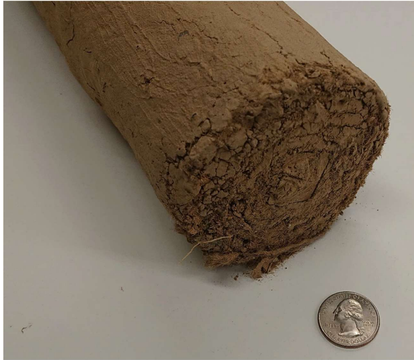
Figure 4: Mudroll cross section, with quarter for scale
