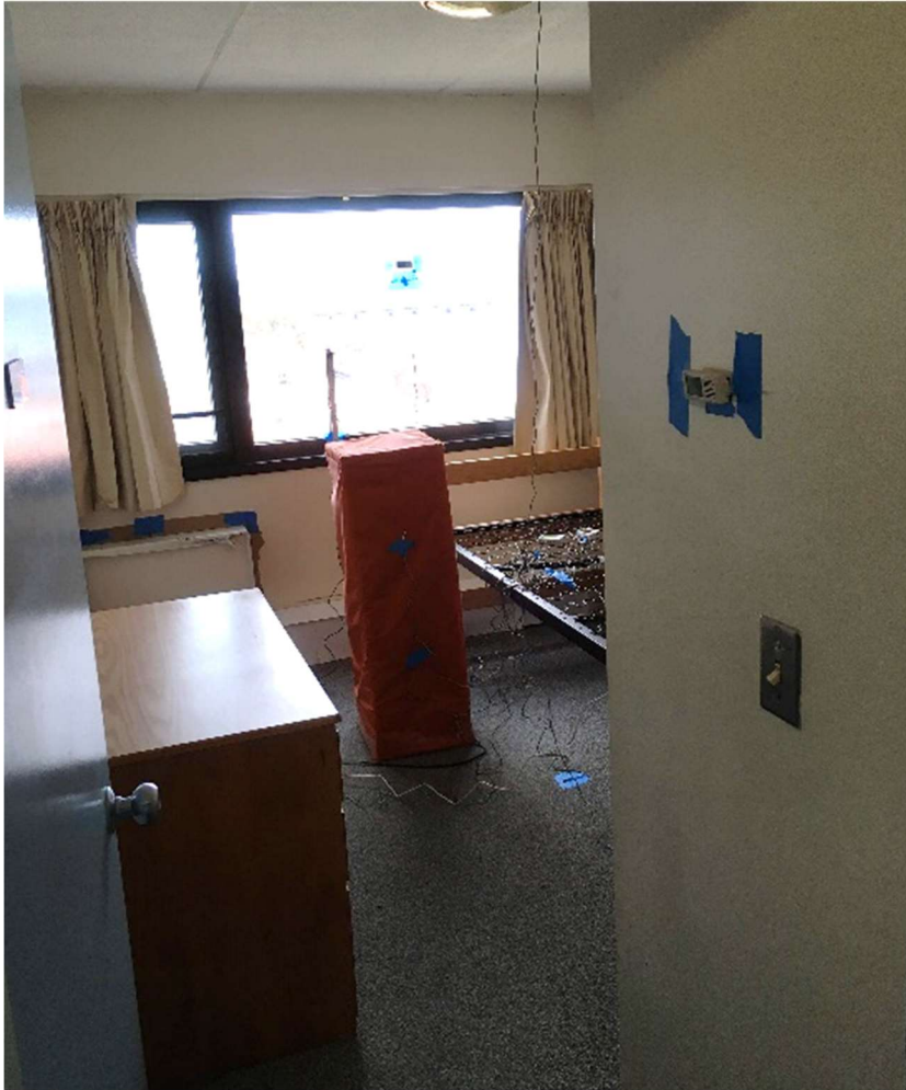
Figure 80: Workspace 1- A complete view of the room from near the door; also shown is a thermocouple sensor near the thermostat position on the wall to the right
