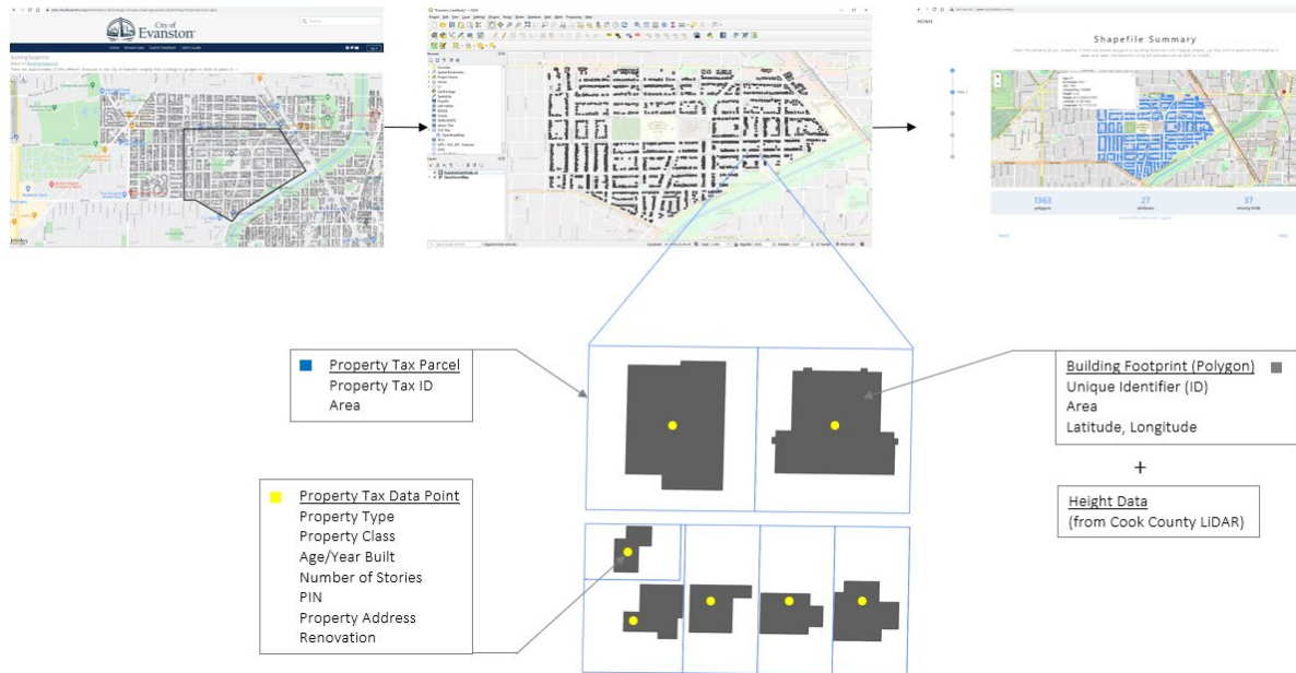
Figure 4-4. Building footprint GIS file retrieved from the City of Evanston’s open data platform (top left), opened in QGIS for processing (top centre), and loaded into UBEM.io (top right), as well as the spatial structure and datasets of the file (bottom).
