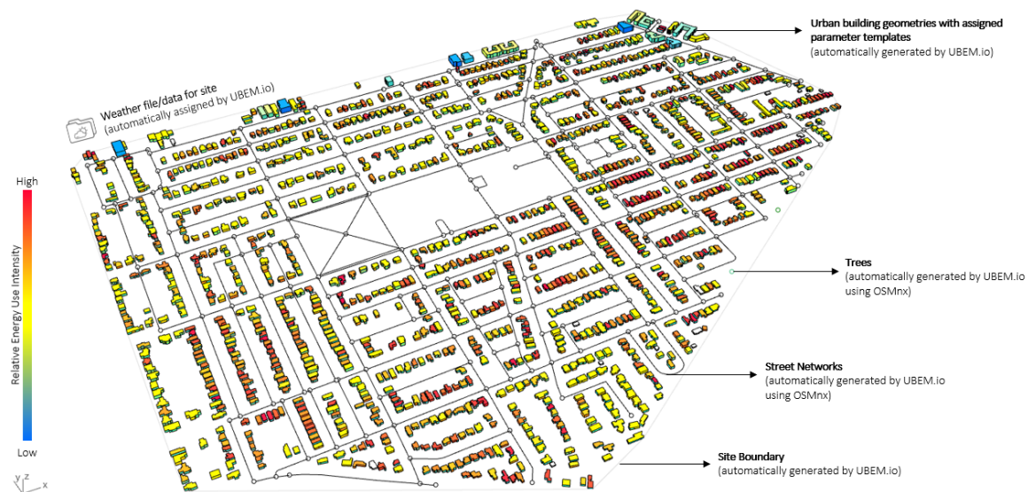
Figure 4-5. Base UBEM generated using UBEM.io’s urban model generator after the simulation is completed.
