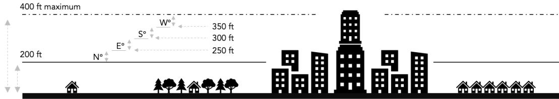
Figure 3-7: Graphic of proposed altitude stratification protocol for UAV-LMD.
