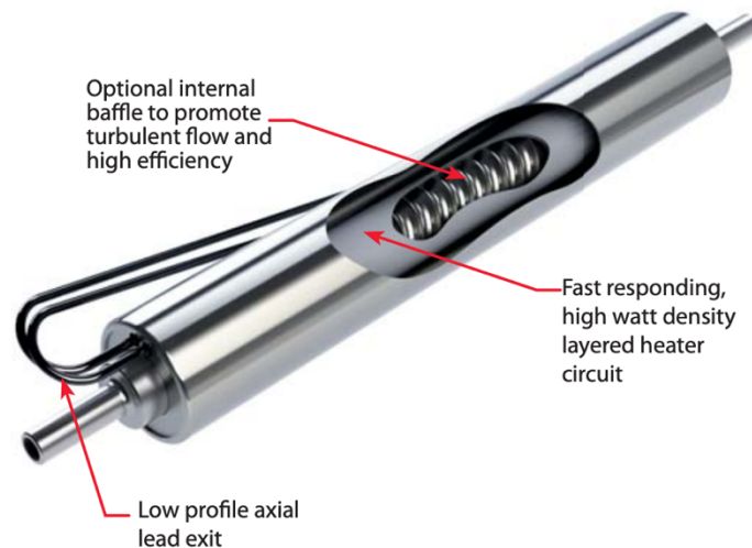
Figure 90: In-line electrical preheater to increase gas temperature to SOE setpoint (Watlow FLUENT Heater).
