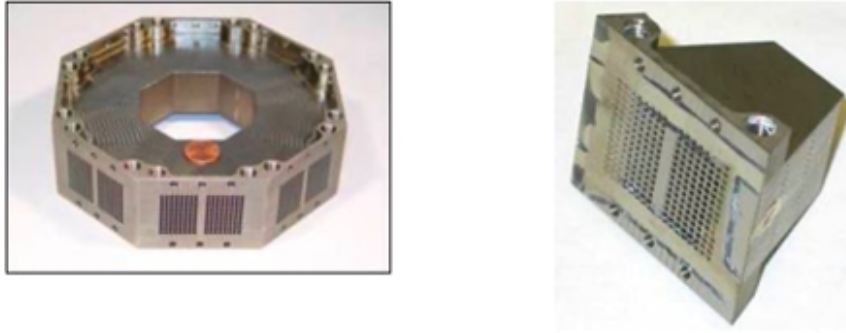
Figure 79: Titanium 8-cell CO 2 sorption pump at TRL-4 from Battelle [142]
