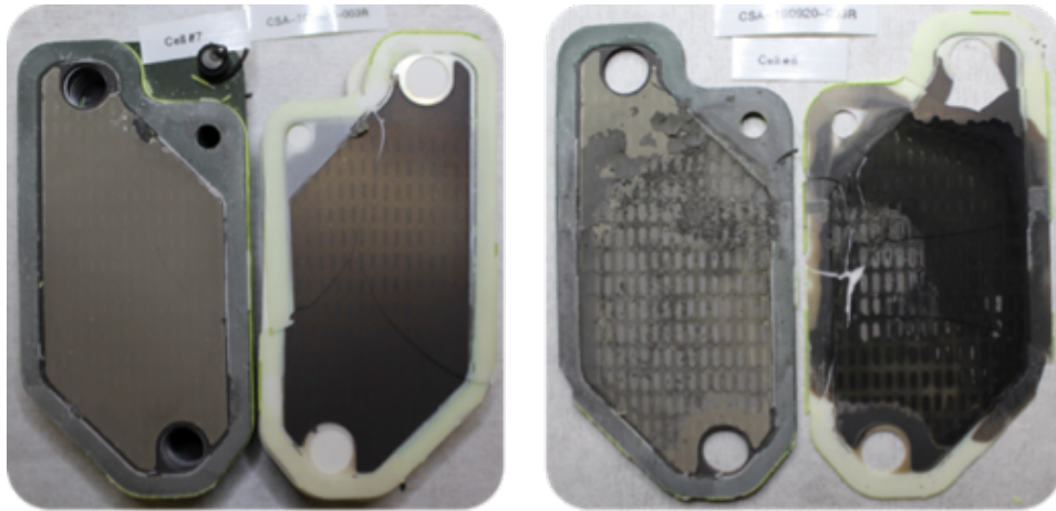
Figure 29: A comparison of a non-coked SOE cell (left) to a cell that experienced coking (right).
