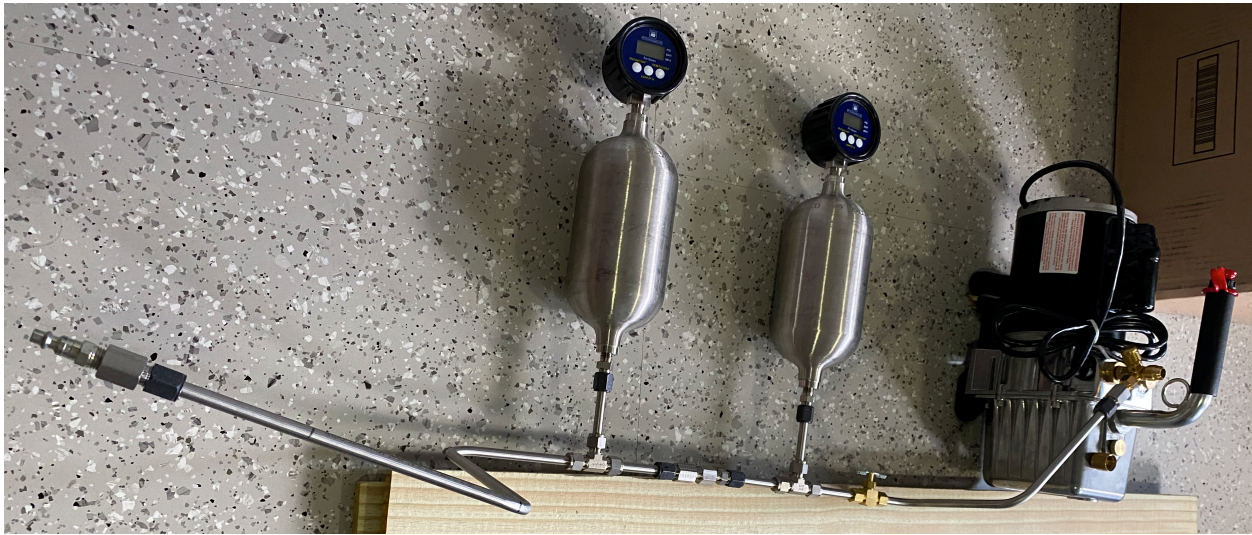
Figure 112: Pneumatics system equipment used in low-pressure SOE tests at OxEon Energy
