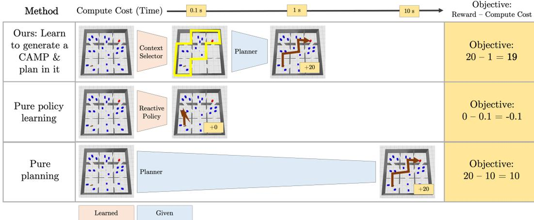
Figure 4-2: Three approaches to solving an MDP. Given a task, our approach (top row) applies its learned context selector to generate a CAMP, then plans in this CAMP to get a policy. Our approach often achieves higher reward than pure policy learning (middle row), and lower computational cost than pure planning (bottom row), leading to a good objective value (right; uses  $\lambda = 1$  in Equation 4.1).
