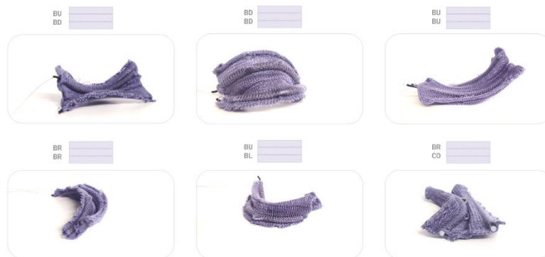
Figure 31. first prototype studies with bending and contracting pneumatics.
