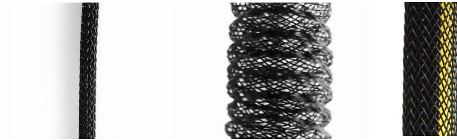
Figure 11. type of braided sleeves used - from left to right: regular braid, post-processed braid for extensible pneumatic, braid with rigid material insert for bending pneumatic.
