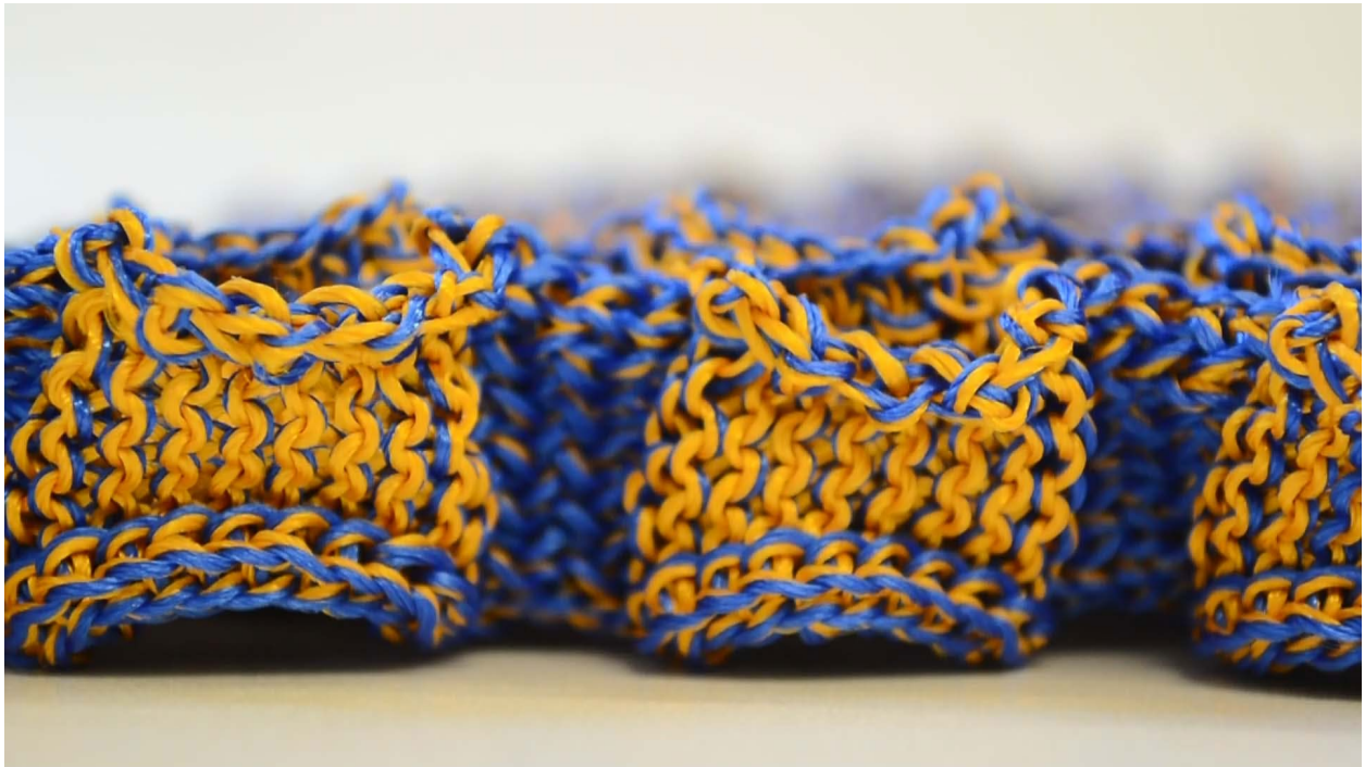
Figure 40. varying cross section of knit, deep cross section when inactive, shallow cross section when active.
