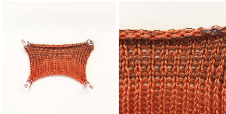
Figure 19. close up of knit sample with conductive yarn.
