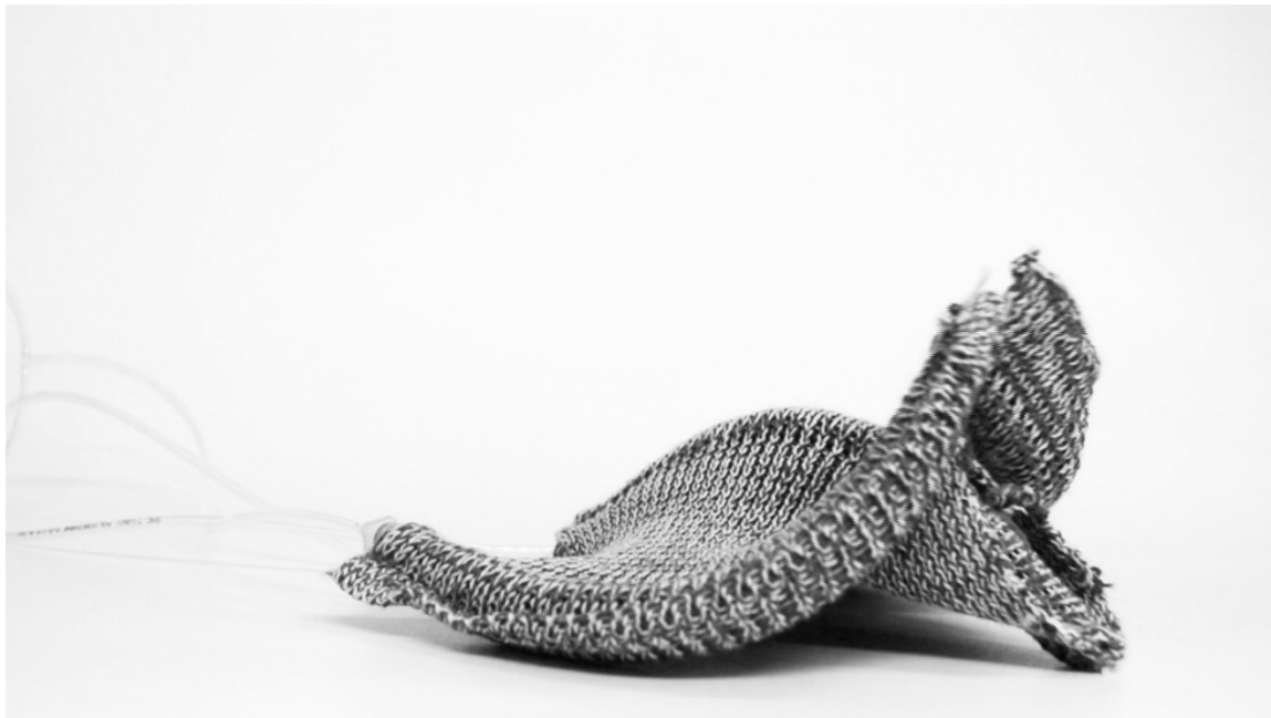
Figure 35. combination of bending and extending pneumatics.
