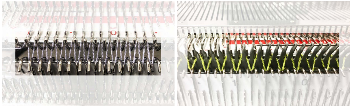
Figure 21. left: initial cast-on process, right: cast-on comb while wire is being inserted.
