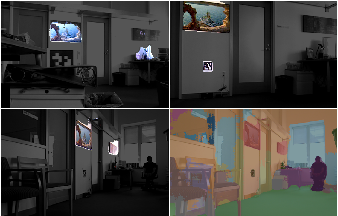
Figure 8-22: Foveation, see Section 7.4.2, Fig. 7-8, and Pixel-wise segmentation, using SegNet [9]: Three keyframe SLAM-aware images recovered through a foveate query. Bottom right shows a repeat image but with segmentation color palette mask overlay. The images show a common scene separated by hours from actual events, and shows how an independent process may now manipulate the persistent database centralized factor graph to introduce new loop closure constraints based on object detections of the painting. The figures also shows a missed painting detection in the top images, which can be used to improve training of the detection and classification algorithms. This figure was modified from [64].
