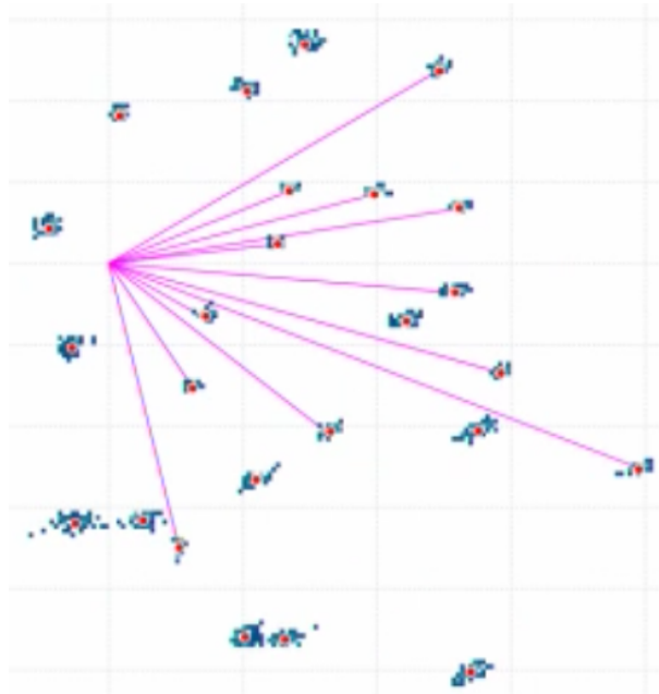
Figure 8-14: Single snapshot view of front-end processing for the Victoria Park outdoor dataset, showing laser scanner detections and tracked features. Tracking of objects is performed with inverse odometry and a Bayesian filter — using Sudderth & Ihler et al.’s multi-scale Gibbs sampling strategy on kernel density estimates [218] — to assign non-overlapping feature IDs while detections are in the field of view. The vehicle is traveling from left to right.
