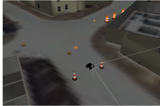
(b) The world state after the robot completed its goal. The initial command “Drive to the cone” was ambiguous. The inverse semantics process generated the disambiguating question “Did you mean the far cone or the right cone?”. The reply “the far cone” produced the illustrated and achieved goal state.
