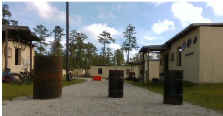
Figure 13. A robot field experiment scenario of a street market with various realistic entities, such as bicycles, shops, motor bikes, fruit stands, among others. The perspective is captured from a camera mounted on the front of a Clearpath Husky A200 Unmanned Ground Vehicle. Prominently displayed are three barrels directly in front of the robot.
