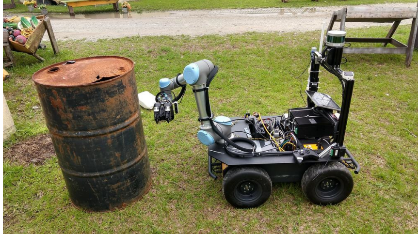
Figure 7. Experiment demonstrating the deliberate interactive estimation with physical interaction. The Husky robot with a UR5 arm estimates the latent semantic attribute “emptiness” by pushing the barrel.
