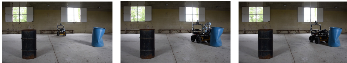
(a) The robot is initially provided with the statements “the leftmost barrel is full” and “the rightmost barrel is full”. (b) The robot deliberately interacts with the barrel to the robot’s left given the robot instruction “push the leftmost barrel”. (c) The robot states “the fact the leftmost barrel is full is inconsistent with world model” after estimating the semantic state as being inconsistent with the world model. The robot also internally updates its representation of that object.
