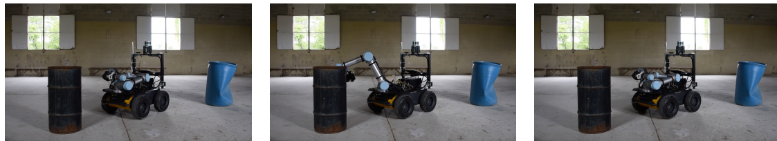
(d) The robot is provided with the instruction “push the full barrel” which is now ambiguous because after interactive estimation it no longer considers “the leftmost barrel” as being full. (e) The robot deliberately interacts with the object originally identified as “the rightmost barrel”. (f) The robot finds that the human-provided description is consistent with the interactive measurement of the object and provides no report back to the operator at the conclusion of the action.
