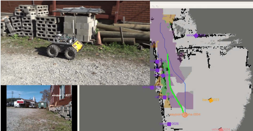
(c) Illustration of the two distinct paths generated by the different planners when navigating to the waypoint alpha. The blue trajectory comes from the shortest path, obstacle avoidance planner, and the green trajectory is generated by the learned behavior for terrain-aware planning.
