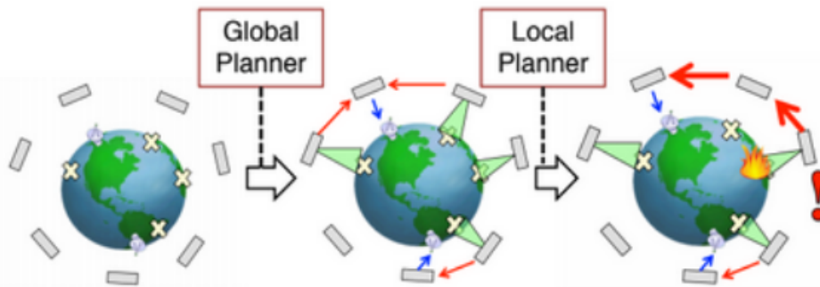
Fig. 1 A coordinated response of a constellation to an unexpected disaster, showcasing the passing of plans and data to rapidly image new data and downlink it. [11]
