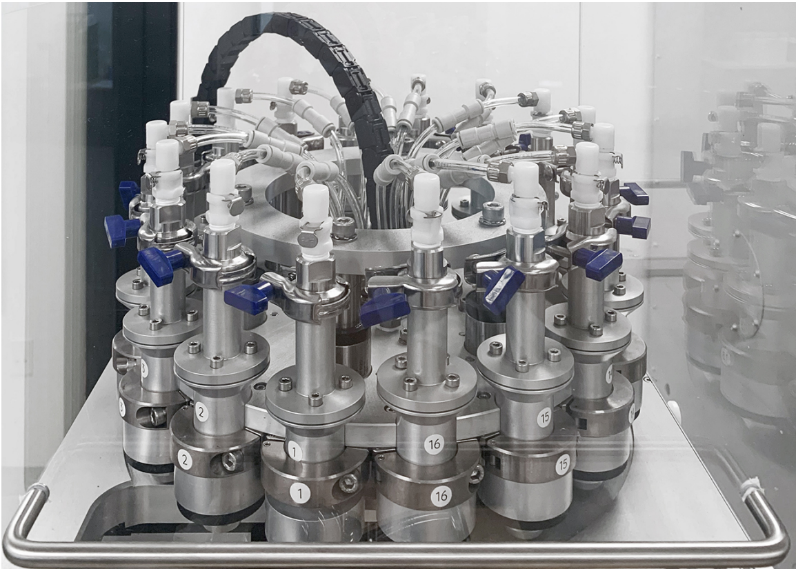
Figure 2-3: Alloy Development Feeder, designed for materials development and research (Credit: FormAlloy)
