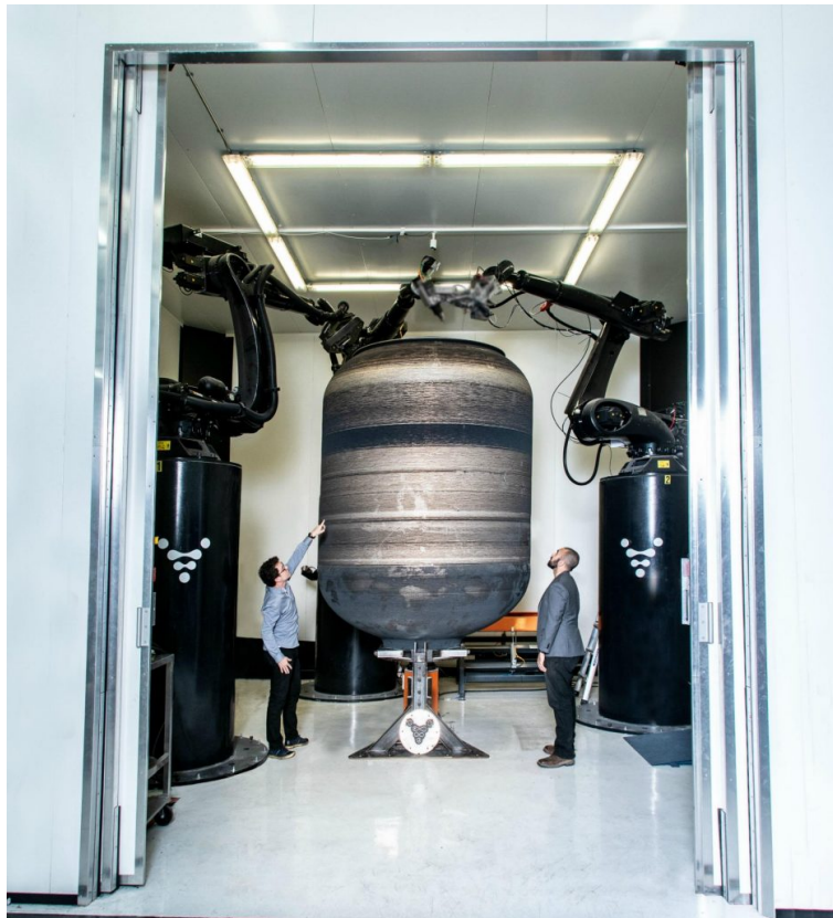
Figure 2-6: Fuel Tank Built by Stargate[14]
