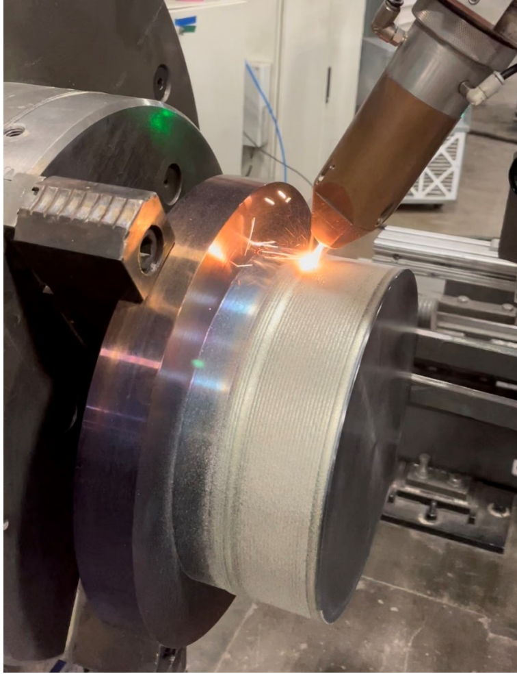
Figure 3-1: Photo Taken at ACT During the East Granby Site Visit - Surface Cladding in Progress
