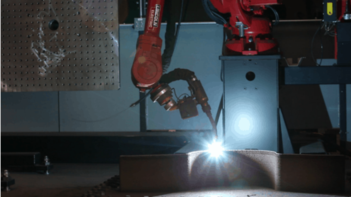
Figure 3-2: Lincoln Electric - Wire Arc Additive Manufacturing Machine[4]
