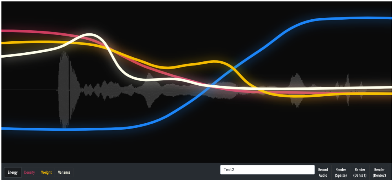
Figure 1: Prototype interface for the Sound Sketchpad. The grey waveform represents the input audio sketch, which the user supplies (for example, through vocalization) as a "template" for the resulting composition. Each colored contour represents a parameter that can be varied over the course of the sketch to shape the qualities of the output.
