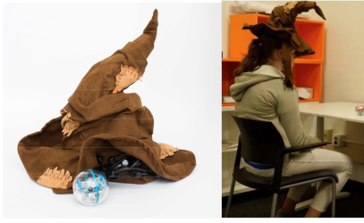
Figure 1: Left: The Thinking Cap system incorporating a Sorting Hat, an EEG headset as well as speakers inside of hat (not visible on this image). The image also features a small Sphero robot used in this study. This setup was used in FULL condition of our study. Right: Participant undergoing Stage 3 of the study.
