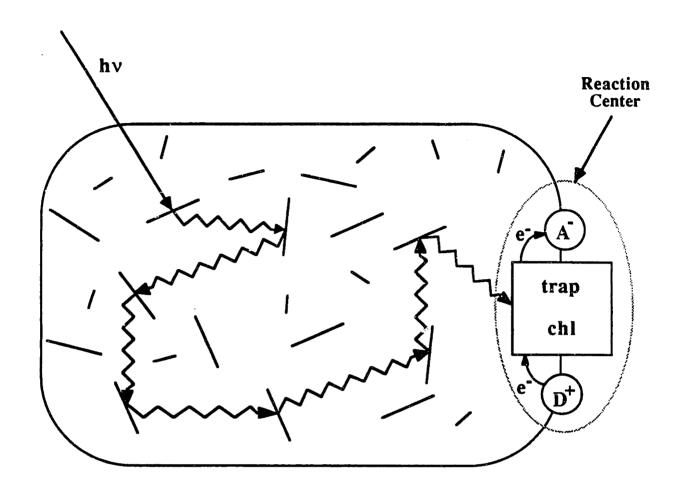
Figure 1. Schematic of the light harvesting unit in a photosynthetic cell where a photon  $(h\nu)$  is absorbed and transferred to the trap chlorophyll. The acceptor (A) receives the excited electron from the trap which is then reduced by a suitable electron donor (D). (Adapted from Nobel, 1970).
