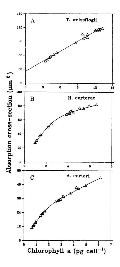
for chl a at 675 nm while the fluorescence measurements are for blue excitation, but the purpose here is only to compare the trends. The similarity of the trends between Figure 18 and Figures 3, 7 and 11 supports the hypothesis that changes in absorption cross-section due to changes in pigment content and cell size are important in predicting fluorescence intensity.
