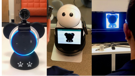
Fig. 2: Left to right: Home agent, Home agent migrating to receptionist robot, Home agent migrating to waiting room assistant.
