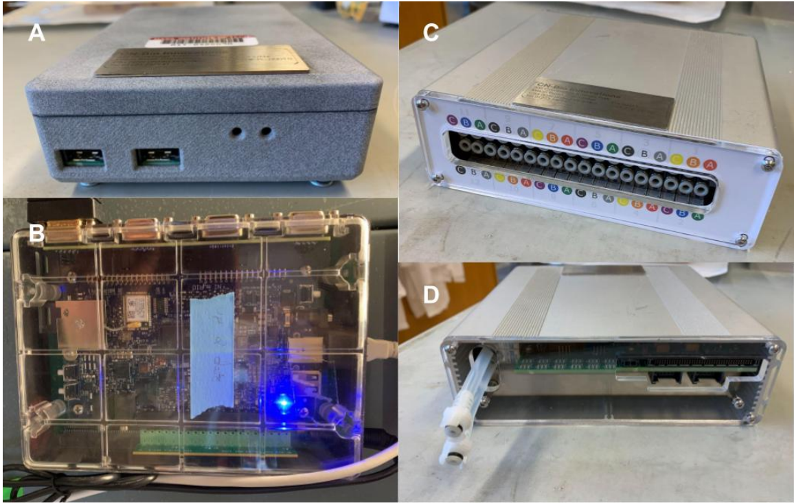
Figure 3-1: The two units that make up the standard pump control system made by CN-Bio. A) The unit that contains the controller hardware. B) An earlier version of the unit containing the controller hardware in which the hardware is visible through a clear lid. C and D) The unit that contains the pneumatic and associated electronic hardware.
