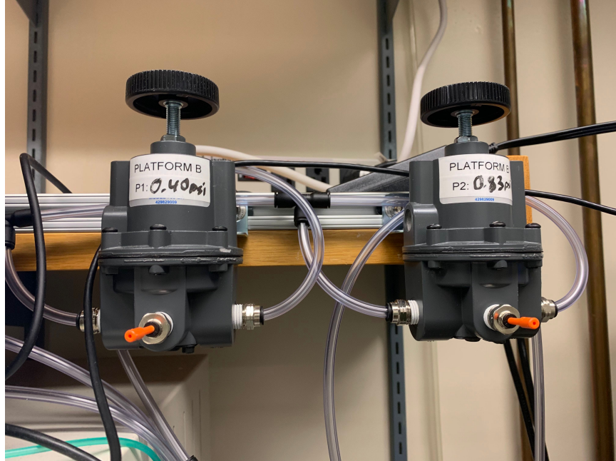
Figure 7-1: Two pressure regulators (2-5 psi) mounted in the incubator room. These pressure regulators are used to control the pressure drop across the gel compartment in the EndoChip by acting as the inputs to the two on-chip back pressure regulators.
