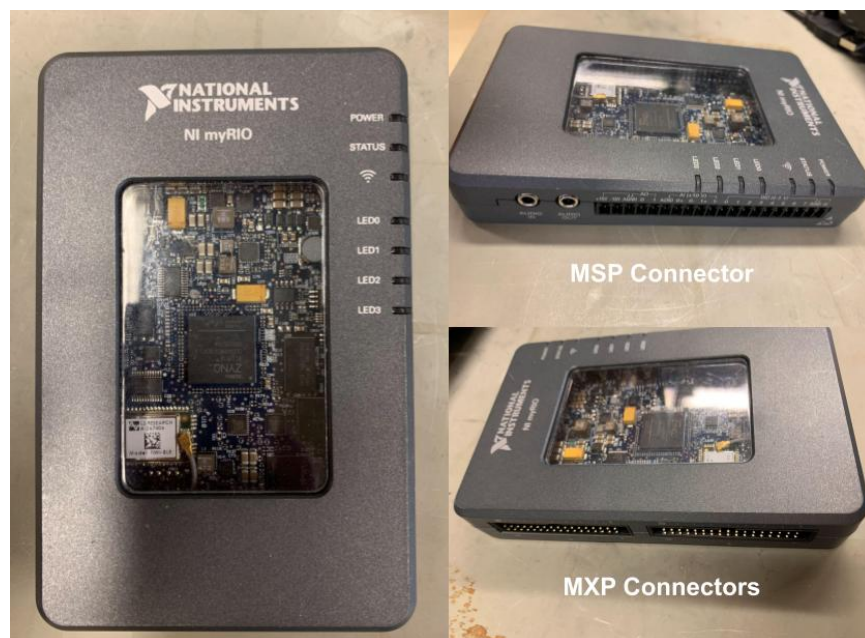
Figure 3-12: An NI myRIO-1900 with the MSP and MXP connectors labeled.
