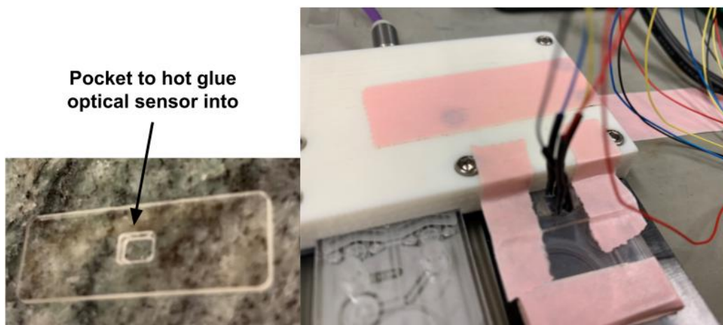
Figure 6-13: The machined optical sensor holder. The pocket depth ensures the sensor is located 0.6 mm above the surface of the chip. The holder is the width of a chip and the sensor pocket is located such that when the edges are aligned with the edges of the chip and the manifold, the sensor is centered above the pump chamber. The optical sensor is secured using hot glue.
