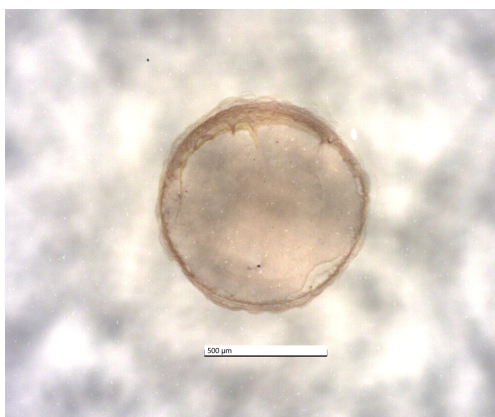
(d) Nanointegris IsoSol-S100 creates a relatively uniform dot, despite the coffee ring effect that can be seen.
