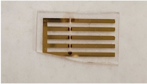
(a) Gold electrode for conductivity testing. (b) Printed CNT sample on gold electrode
