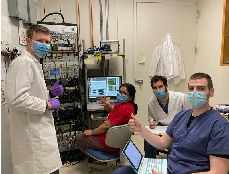
Figure 6-1: From left to right: the author, Annesya, Lukas, and Chris. Behind me an equipment rack connected to the soundproof room is visible, featuring a signal generator, oscilloscope, audio power amplifier, laser doppler vibrometer, and tunable analog antialiasing filters. Annesya is operating an National Instruments PXI running custom measurement software.
