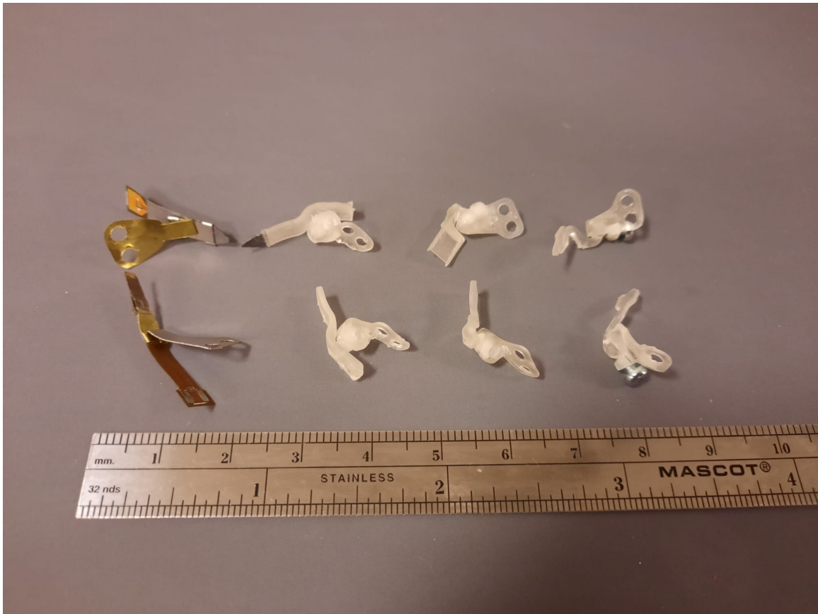
Figure 5-4: A list of prototype platform designs with initial sheet metal designs on the left and improved ball joint designs to the right.
