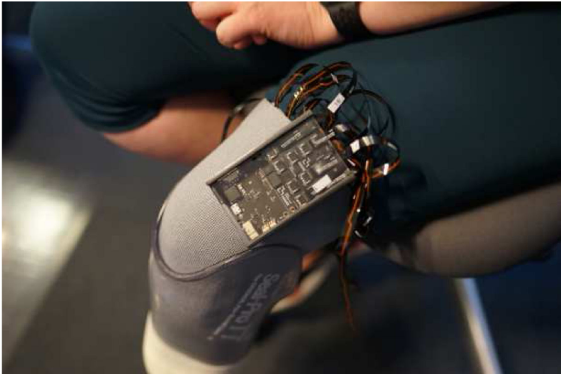
Fig. 9. Example use case of the embedded 16-channel sEMG acquisition and processing platform. The sEMG system is connected to the 16 electrodes as configured in Fig. 8f. This setup does not represent the actual instrumentation setup of the Experiment B, which only instrumented the four muscles of the AMI muscle pairs.
