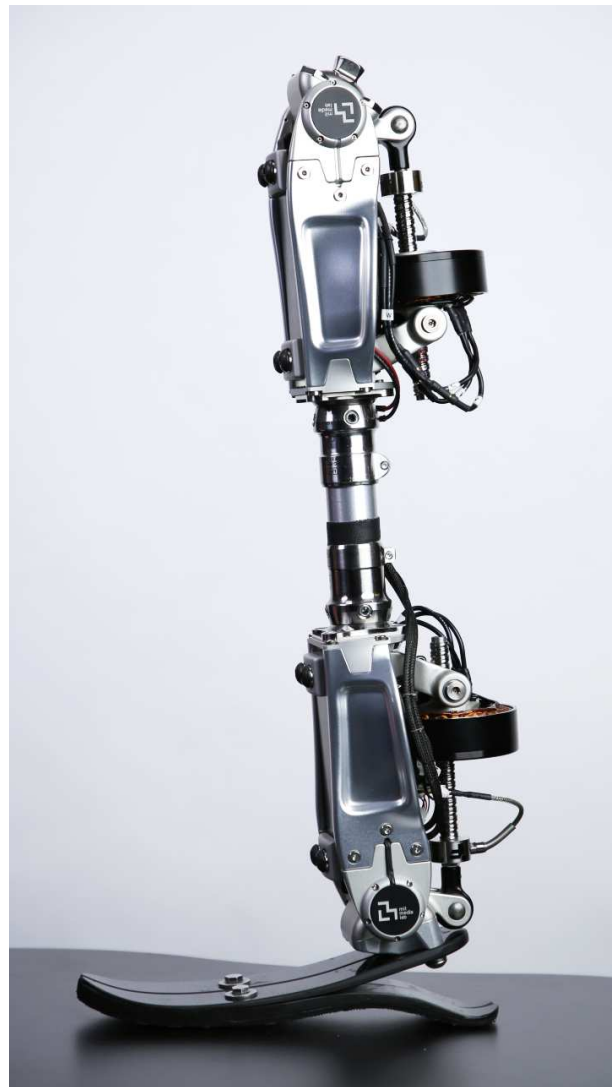
Fig. 1. The TF8 Actuator is designed to operate as either a knee or ankle powered prosthesis. Shown here are two TF8 actuators stacked into a combined powered knee-ankle prosthesis.
