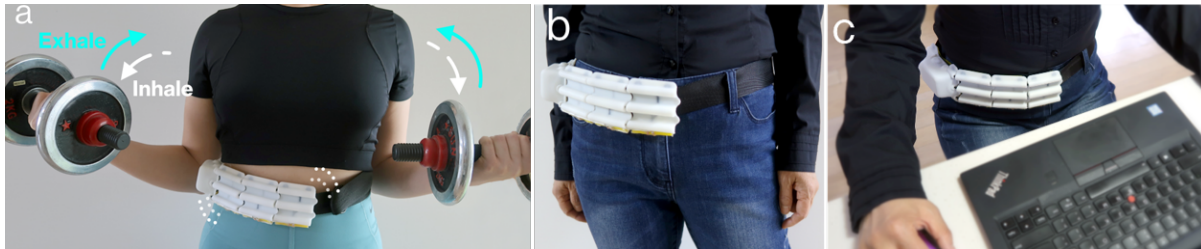
Fig. 22. Application scenarios when the pneumatic-haptic device around waist area (a) for breathing rate and phasing (when to exhale/inhale for how long) guidance during weightlifting, in this case, bicep curl. (b) the device on a waist-belt (c) for stress relief during a office work.
