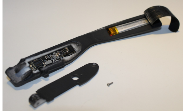
Fig. 16. Battery Placement in Captivate's Arm
