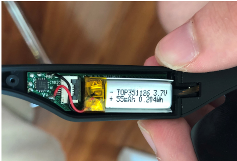
Fig. 15. One Sided Commercial Battery Design of Smart Eye-Wear
