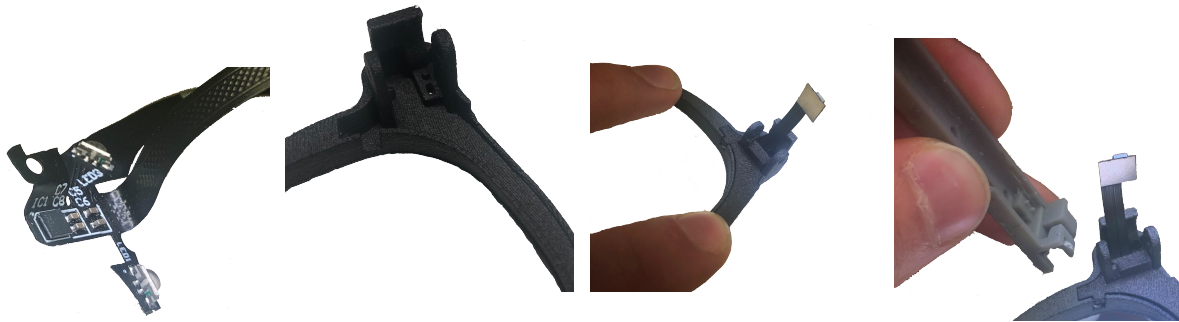
Fig. 9. Pre-bent Flex Circuitry Fig. 10. Inside of Front Housing Fig. 11. Sealed Front Housing with Flex Circuit Integrated Fig. 12. Adding a Side Leg
