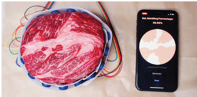
Figure 10: An EIT device for sensing biological tissue, i.e. the percentage of fat and lean tissue in the sample.
