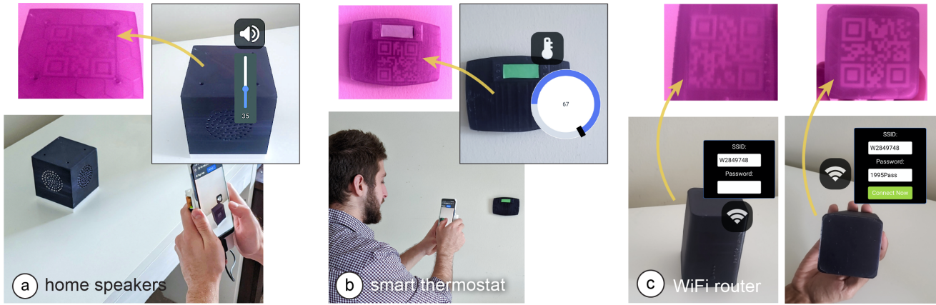
Figure 7: Controlling appliances using a mobile AR application. The user points at (a) the home speakers to adjust its volume, and the (b) thermostat to adjust the temperature. The infrared camera in the phone’s case identifies the appliances by reading the embedded QR codes. (c) Pairing a phone with a WiFi router, whose SSID is visible from all sides but the password is visible only from its bottom.
