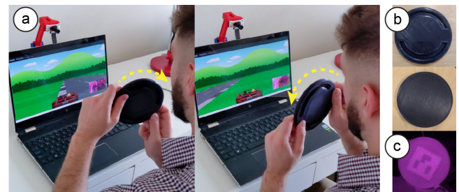
Figure 9: Using passive objects (a) as a game controller. (b) This wheel is black under visible light and has no electronic components. (c) The fiducial marker embedded inside is only visible to an infrared camera.
