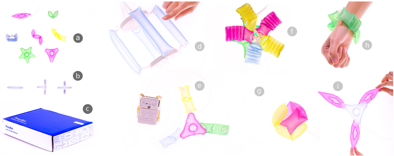
Figure 1: The PneuBots kit features (a) 7 inflatable modules, (b) 3 types of pneumatic connectors, and (c) a custom-designed package. Some of the dynamic assemblies possible with PneuBots, in combination with FlowIO Platform, include (d) a rolling robot, (e, f) different artistic designs, (g) a self-assembled ball, (h) a haptic bracelet, and (i) an interactive flower.
