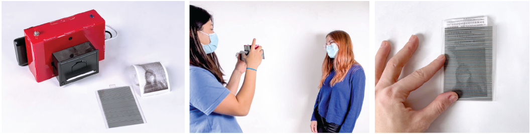
Fig. 1. KineCAM is an instant camera-inspired device that allows users to capture and fabricate animated photographs, in the form of kinegrams, on the spot. (© Ticha Sethapakdi. Photo: Thanh Nguyen, 2021)
