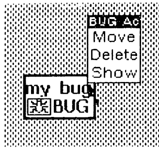
Figure 2: A link to the my bug object in Figure ?. The top line in the link is the value of the Name: field. The icon at the bottom left is the icon for the BUG template. The bottom line is the template name. Clicking the mouse with the right button on the link produces the popped up action menu as shown. Move moves the link to a user-selected position on the screen. Delete deletes the link. Show displays the object of this link.
