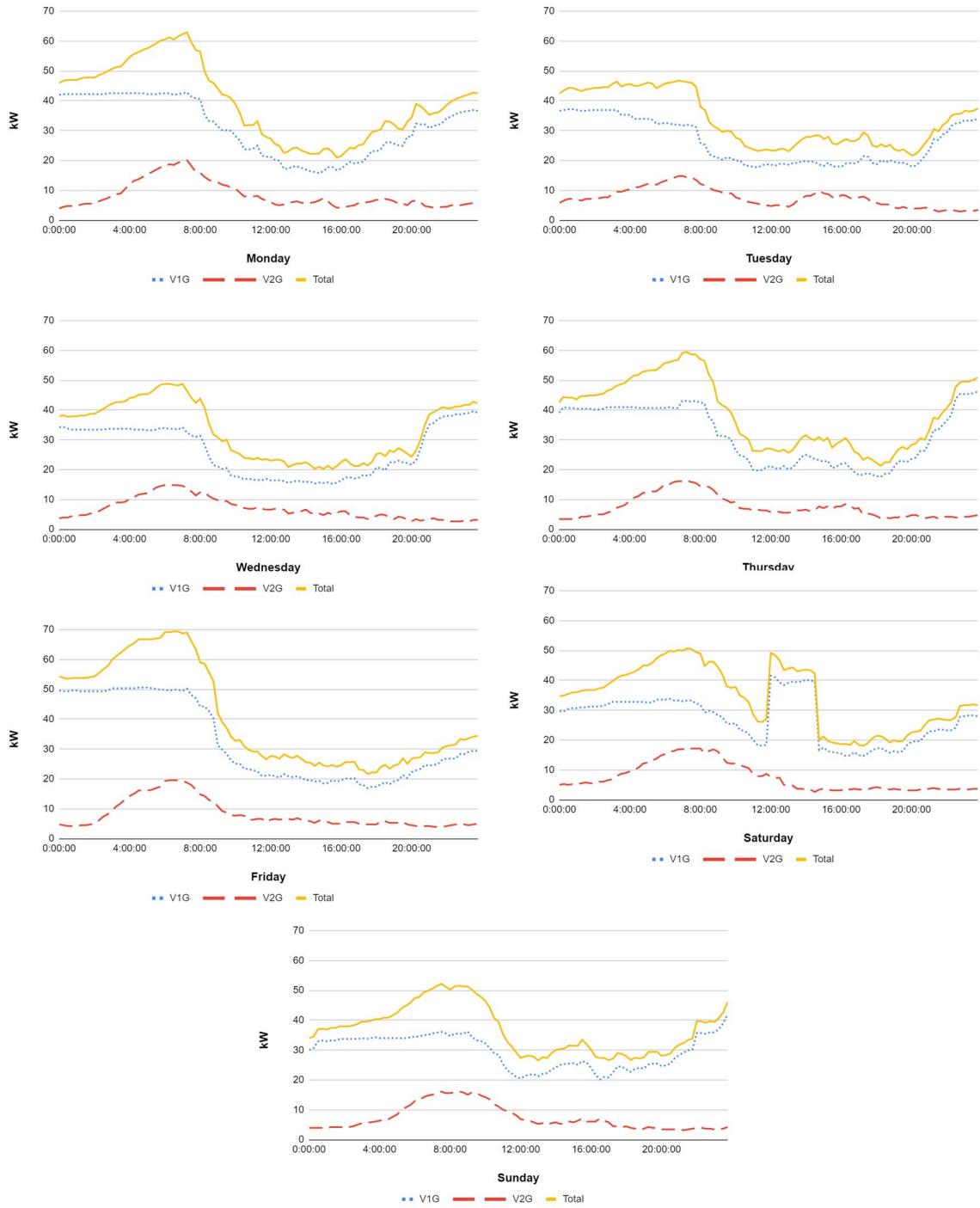
Figure A-1: Average power available, power consumed, and dispatch time for each day of the week
