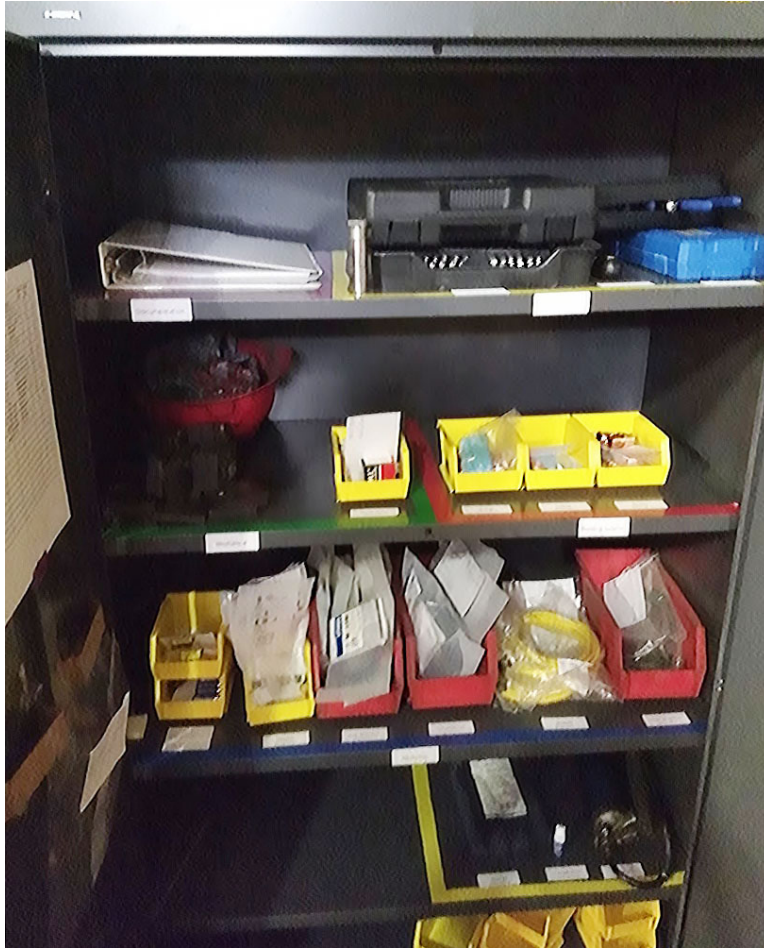
Figure 7-1: A picture of the spare parts cabinets. Visible are the bins containing each unique spare part, with labels applied to the cabinet and reorder cards inside the bins. At the top left is the documentation binder, and at top right are specific tools for the machine. At far left is an listing of the parts and quantities that should be present when inventory is counted.
