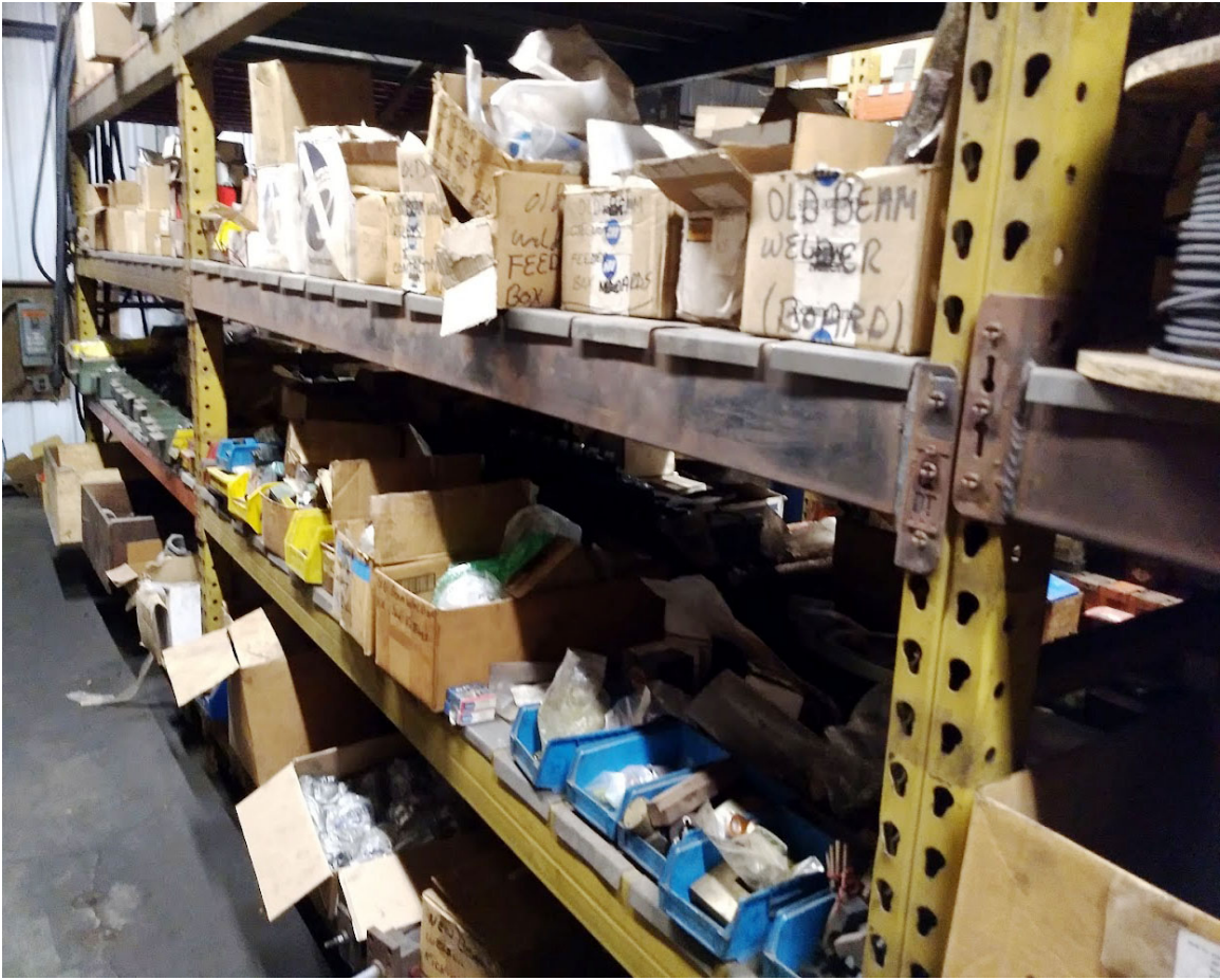
Figure 5-3: Shelves in the spare parts room, labeled A in figure 2-6. Cardboard boxes containing spare parts are stacked on pallet racking. Some boxes are labeled with permanent markets, but there are no part numbers. Many parts are covered in a layer of dust. Parts are not counted regularly.
