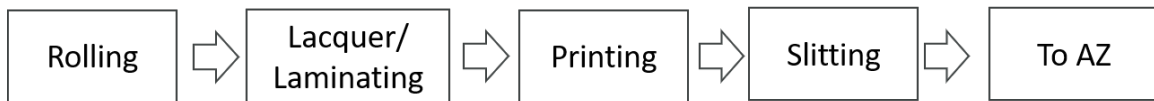
Figure 2-2: Example of foil making process. In this example there are a few key steps such a rolling the material, applying lacquer or paint depending on the specifications, and then slitting the material to size to ultimately be distributed to the buyer’s site.
